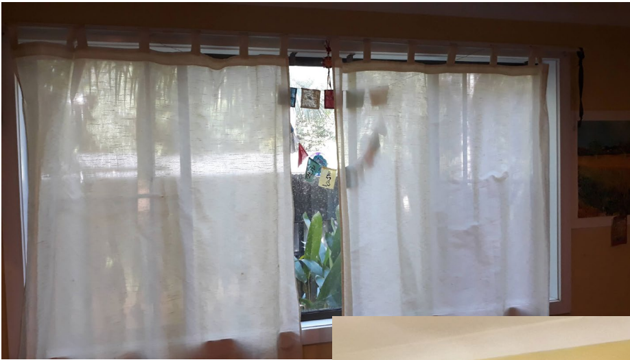
The original curtains (above) were thin and sheer and did very little to retain heat. The new curtains (right) are much thicker, with a thermal lining.
